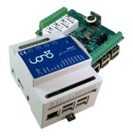
Iono Pi is an extremely versatile I/O module that combines several digital and analog input lines, support for standard interfaces like 1-Wire and Wiegand and power relay outputs, typical of modern PLCs, with the powerful 1.2GHz quad-core ARM Cortex-A53 64-bit processor of the Raspberry Pi 3.
